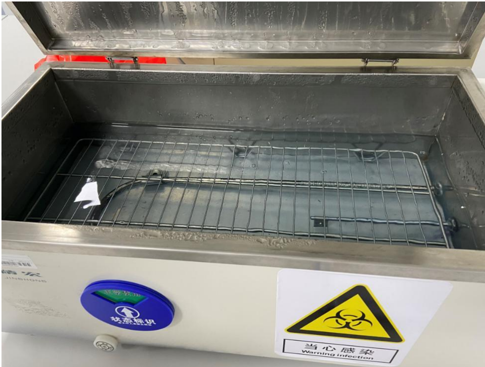
Picture 2-2 Laboratory Water Bath for Sample Inactivation
